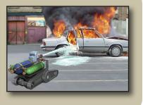
The iRobot Warrior is a powerful and rugged robot that can carry greater than 150 lb payloads, travel through rough terrain and climb stairs with heavy loads. The robot's design offers an advanced digital architecture and an extremely sturdy platform to support the weight of heavy payloads, such as firearms and hoses. The Warrior robot will be
